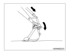
(10) To engage the quick coupler, release the quick coupler button on the right joystick lever.
