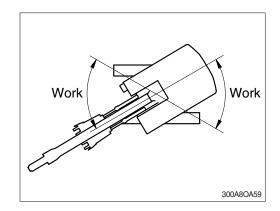
Conversely, if thrust is excessive or breaking is performed with boom of the lower chassis raised as shown, the machine may suddenly tip toward the movement. The breaker body may strike the broken rocks violently resulting in damage.
