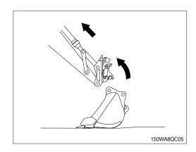
(8) Move the arm (1) and raise it until hook engages the upper pin (2) or interface of attachment.
